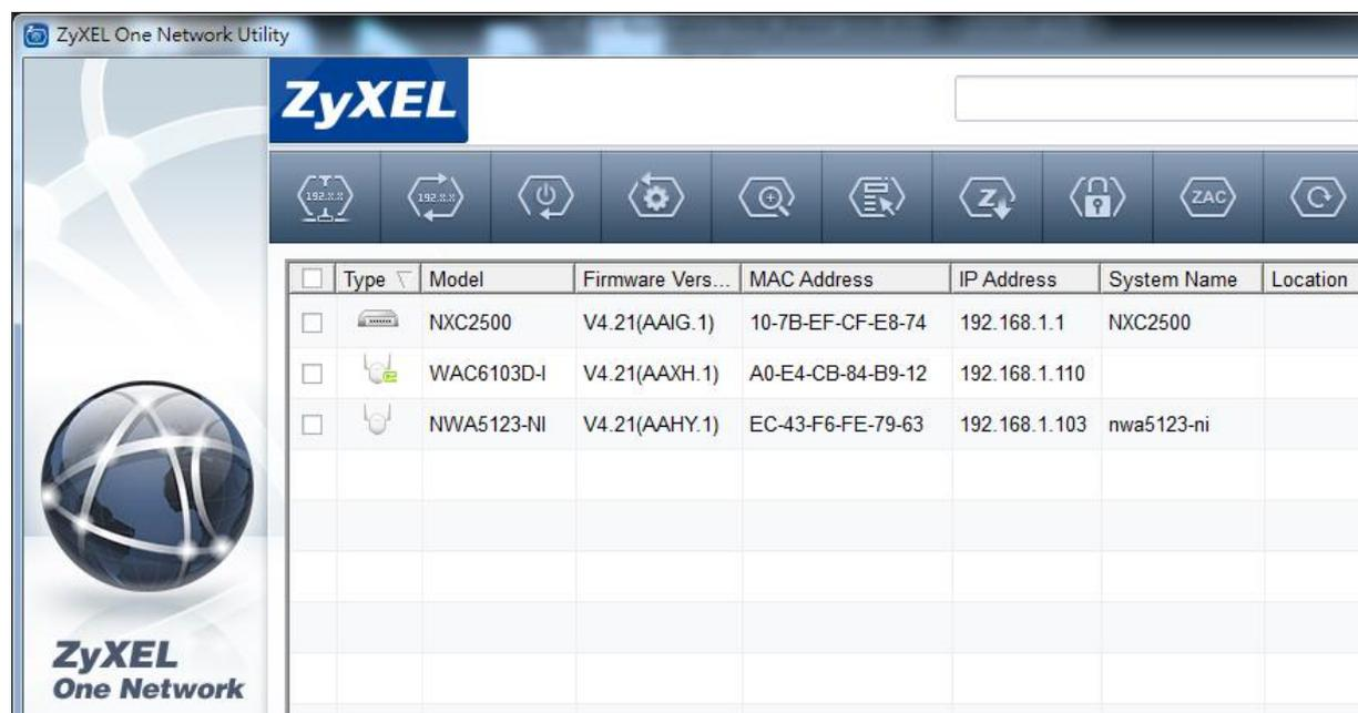
The above screen shows an example of the ZON Utility discovery: one NXC2500, one WAC6103D-I, and one NWA5123-NI. The WAC6103D-I is configured as a managed AP and the NWA5123-NI is configured as a standalone AP. With the new firmware v4.21, you can see that both AP modes can be discovered via the ZON Utility.
