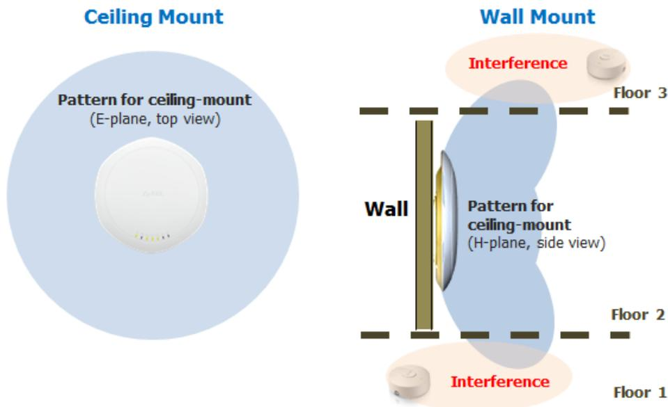
The WAC6103D-I wall-mount pattern focuses the signals to the front end to eliminate interference to other floors.
