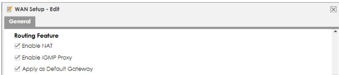
The screenshot shows the 'WAN Setup - Edit' configuration window. The 'General' tab is selected, and the 'Routing Feature' section is expanded. Three options are checked: 'Enable NAT', 'Enable IGMP Proxy', and 'Apply as Default Gateway'.
