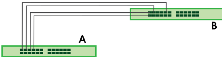
Figure 116 Trunking Example – Physical Connections
