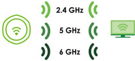
Figure 10 Multi-Link Operation Example
