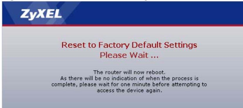
You can also press the **RESET** button on the rear panel to reset the factory defaults of your ZyXEL Device. Refer to [Section 1.7 on page 26](#) for more information on the **RESET** button.
