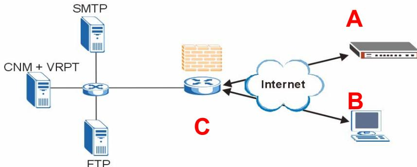
If Vantage CNM is behind a firewall, you must setup firewall rules to allow traffic to flow to/from Vantage CNM to the ZyXEL devices. You must also configure NAT port forwarding to allow the following traffic to be forwarded to Vantage CNM via the following ports:
