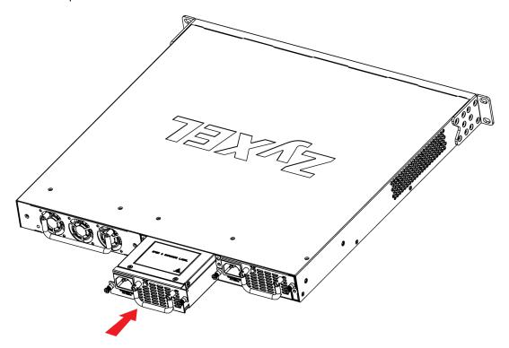
4 Slide the power module into the slot until it makes contact with the backplane and tighten the screws.
