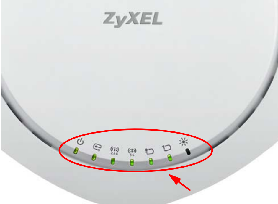
Figure 5 WAC6500 Series LEDs
