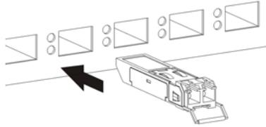
**Figure 5** Connecting the Fiber Optic Cables
