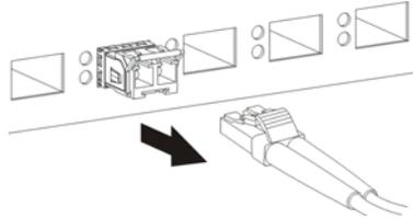
**Figure 7** Opening the Transceiver's Latch Example
