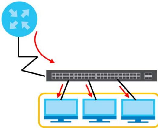
**Figure 96** Static Multicast Forwarding to A Single Port
