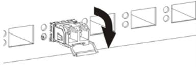
**Figure 18** Transceiver Removal Example
