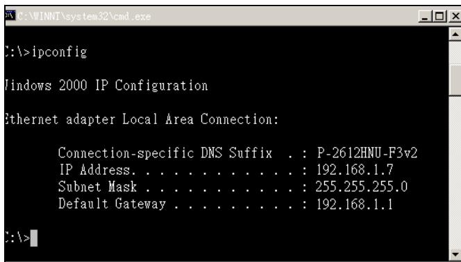
A screenshot of a Windows 2000 Command Prompt window titled 'C:\WINNT\system32\cmd.exe'. The command 'ipconfig' is run, displaying network configuration details for an 'Ethernet adapter Local Area Connection'. The output shows the connection-specific DNS suffix as 'P-2612HNU-F3v2', the IP address as '192.168.1.7', the subnet mask as '255.255.255.0', and the default gateway as '192.168.1.1'.
