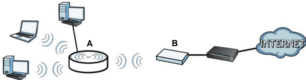
After the WAP6806 and the access point connect, the WAP6806 acquires its IP address from the access point. The clients of the WAP6806 can now surf the Internet.
