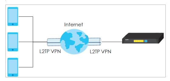
**Figure** VPN2S connect with Mobile through L2TP VPN Tunnel
