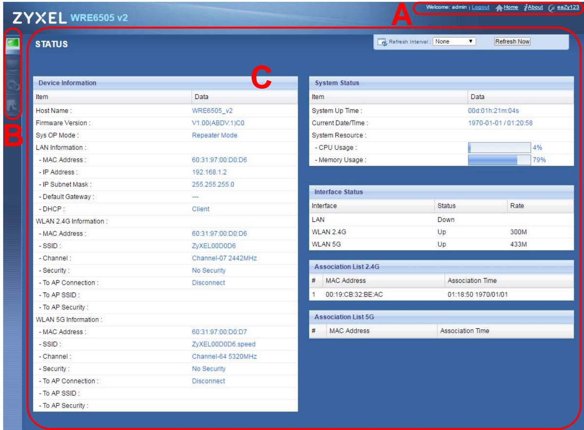
The Web Configurator's main screen is divided into these parts:
