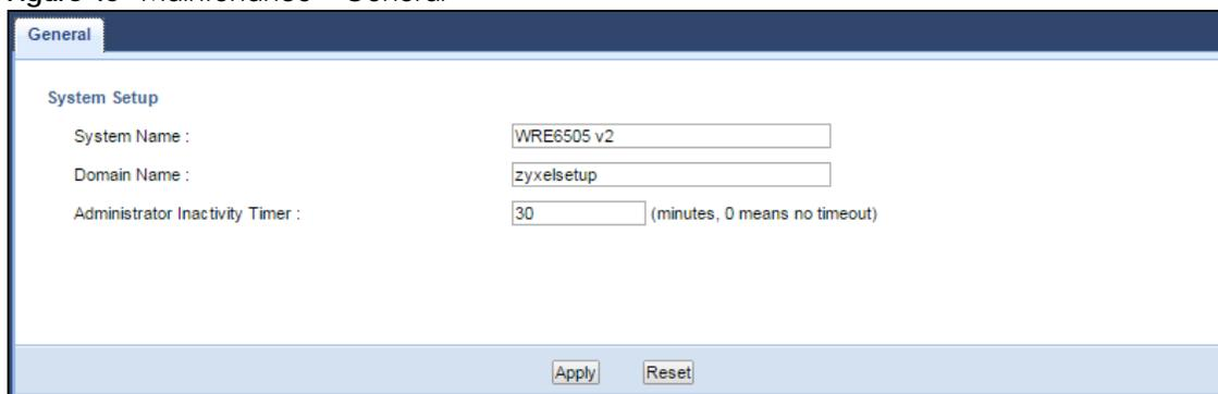
The screenshot shows the 'General' tab of the maintenance screen. Under the 'System Setup' section, there are three input fields: 'System Name' with the value 'WRE6505 v2', 'Domain Name' with the value 'zyxelsetup', and 'Administrator Inactivity Timer' with the value '30'. A note next to the timer field says '(minutes, 0 means no timeout)'. At the bottom of the form are 'Apply' and 'Reset' buttons.
