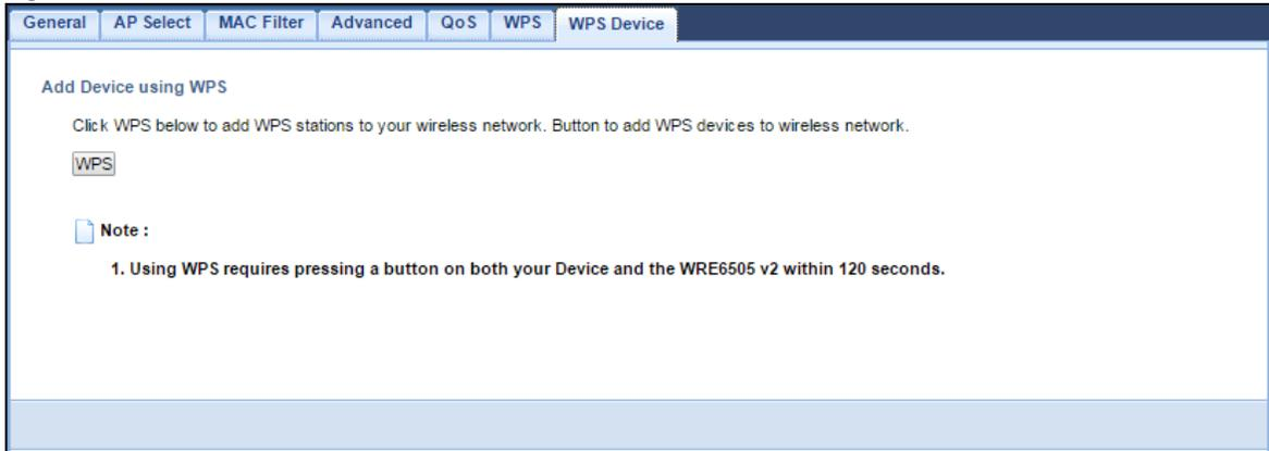
Figure 38 Network &gt; Wireless LAN 2.4G/5G &gt; WPS Device (AP Mode)
