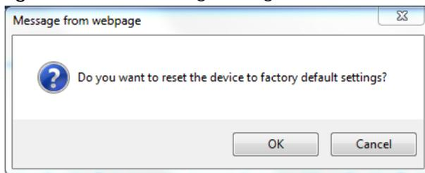
You can also press the **WPS** button (see [Section 1.4 on page 11](#)) on the front panel for more than 10 seconds to reset the factory defaults of your WRE6505 v2. Refer to [Section 1.4 on page 11](#) for more information on the resetting the WRE6505 v2.
