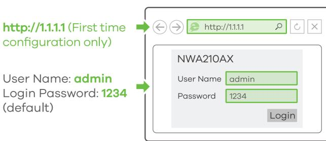
**EN 1-0** From a WiFi enabled computer, search for the NWA210AX's default WiFi network name (**Zyxel-xxxx**, where xxxx is the last four characters of the MAC address) and connect to it.
