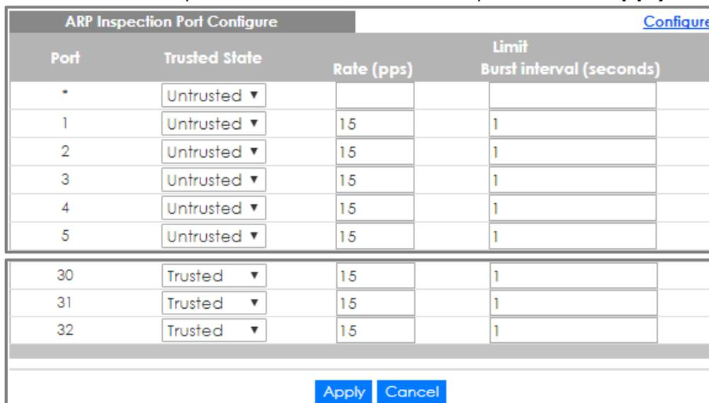
The screenshot shows the 'ARP Inspection Port Configure' table. The table has columns for 'Port', 'Trusted State', 'Rate (pps)', and 'Limit Burst interval (seconds)'. The 'Trusted State' column contains dropdown menus with 'Untrusted' or 'Trusted' selected. The 'Rate (pps)' column contains the value '15'. The 'Limit Burst interval (seconds)' column contains the value '1'. At the bottom of the table, there are 'Apply' and 'Cancel' buttons.
