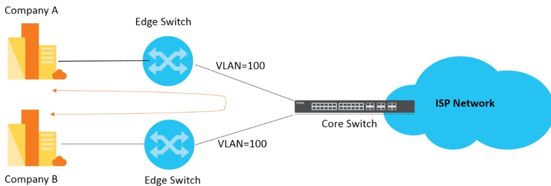
Once VLAN Mapping is configured on edge switches, it can translate customer VLANs of company A and company B to different VLANs respectively. Thus, the traffic will not be forwarded between company A and company B since they are in the different VLANs after processing VLAN translation on edge switches.
