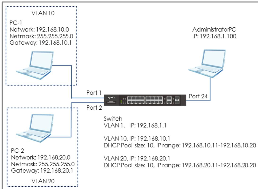
**Figure 11 Perform DHCP service in different VLAN**
