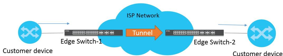
When Edge switch-1 receives Layer-2 protocol packets, it will encapsulate these packets and rewrite their destination MAC addresses with a specific MAC address. All the switches inside the service provider network treat these encapsulated packets as data packets and forward them to the other side. When Edge switch-2 receives these encapsulated packets, it will de-capsulate them and change their destination MAC addresses back to the original one before forwarding them to the destination switch.
