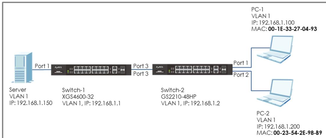
**Figure 20** Configure MAC filter to block unwanted traffic
