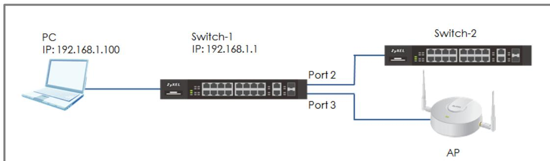
**Figure 5** Configure the port name of the switch
