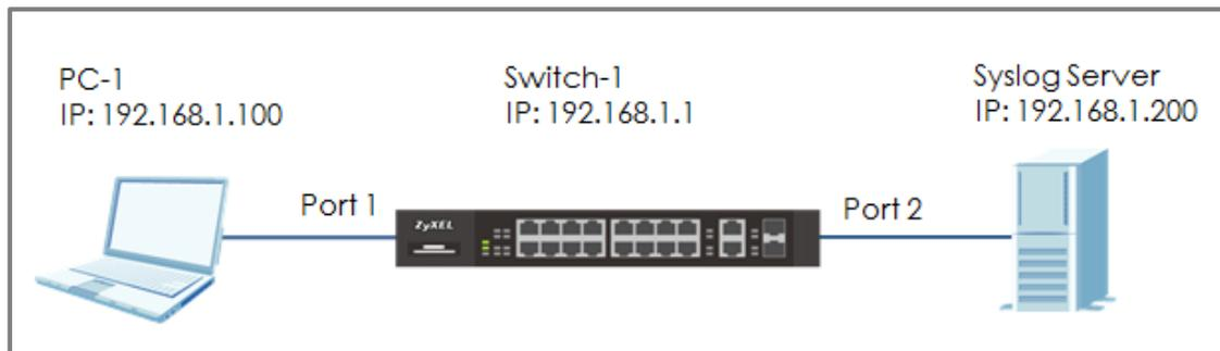
**Figure 4** Upload the syslog automatically to the server
