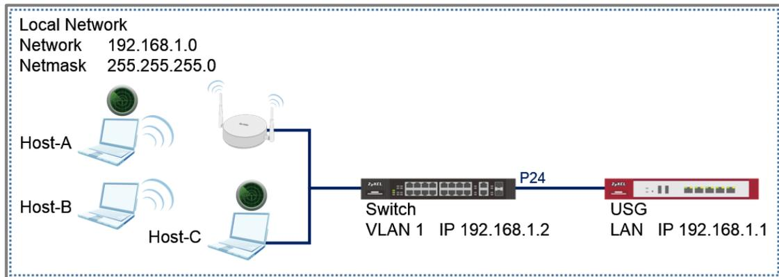
**Figure 21 IP Scanning from Wired and Wireless Devices**
