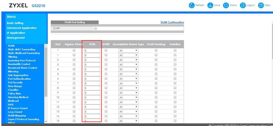
After setting PVID for data packets, next step is to configure “Voice VLAN” feature for the switch to identify the voice packets.
