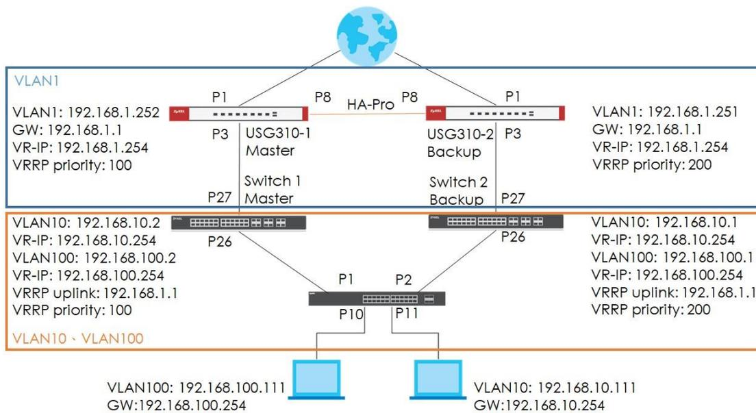
Upon the topology, the normal traffic flow will be like figure 1. However, somehow the gateway device USG310-1 (Master) or the link 1 or 2 has some issues. It will cause all hosts that connected to Switch-1 (Master) not be able to surf the Internet.
