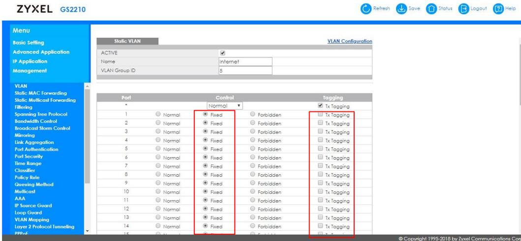
On the uplink port enable Tx Tagging to transmit packets with VLAN tags.
