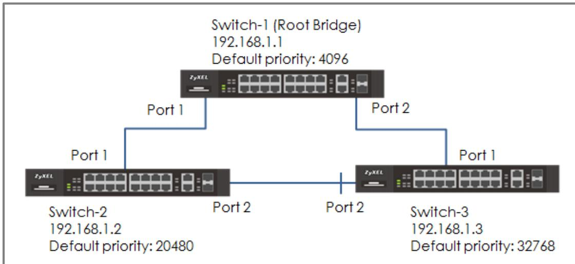
**Figure 13 Configure RSTP in a ring topology**
