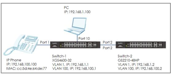
Figure 25 Configure Voice VLAN to separate VOIP traffic from data traffic
