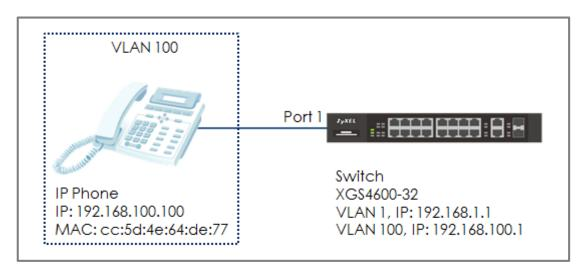
Figure 24 Configure Voice VLAN to separate VOIP traffic from data traffic
