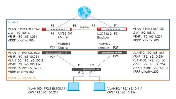
Upon the topology, the normal traffic flow will be like figure 1. However, somehow the gateway device USG310-1 (Master) or the link 1 or 2 has some issues. It will cause all hosts that connected to Switch-1 (Master) not be able to surf the Internet.
