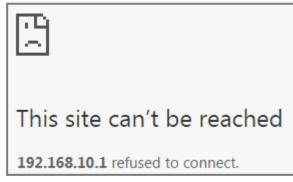
2 The PC-2 (192.168.10.200) is not in the range which is allowed to access the Switch. PC-2 cannot access or ping the switch's management IP address.
