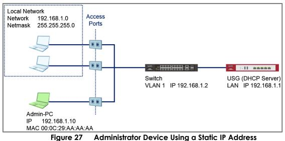
Connected on an Access Port
