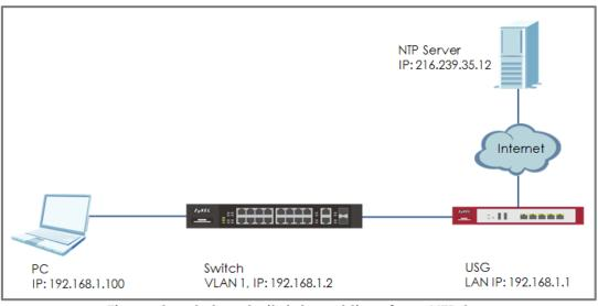
Figure 3 Set up Switch to get time from NTP Server
