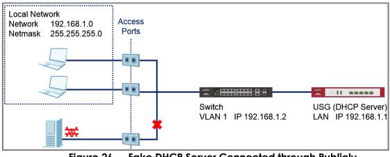
Figure 26 Fake DHCP Server Connected through Publicly Accessible Ports
