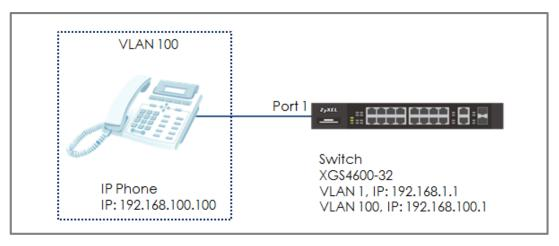
Figure 23 Configure LLDP-MED to assign an IP Phone's VLAN
