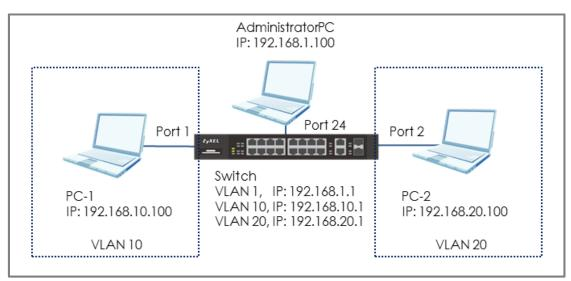
Figure 10 Set up switch to route traffic across VLANs
