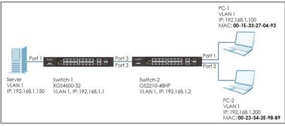
Figure 20 Configure MAC filter to block unwanted traffic
