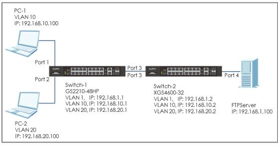
Figure 16 Configure ACL to rate limit VLAN traffic
