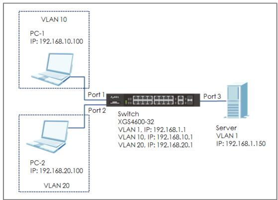
Figure 21 Configure ACL to block unwanted traffic
