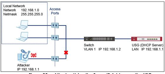
Figure 25 Attacker Using the Same IP Address as the USG
