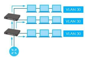
On the Zyxel enterprise switch, we can use the feature "Port Isolation" in Advanced Application -> VLAN -> VLAN Configuration -> VLAN Port Setup to separate traffic between specific ports despite belonging to the same VLAN.
