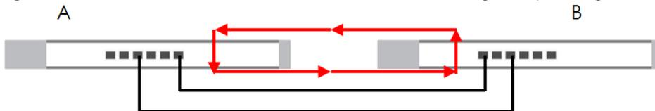
**Loop Detection** allows the Switch to discover a loop if it happens, and create a log. **Loop Prevention** allows the Switch to shut down a port automatically if it discover a loop on that port. See [Section 3.3 on page 19](#) for more information about LEDs.
