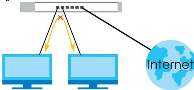
For example, if you have computers grouped together in a VLAN that communicates with servers in other networks. These computers have no need to communicate together, so it is best to block unwanted communication.
