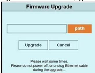
After a successful upload, the system will reboot, and you will need to log into the Switch again.
