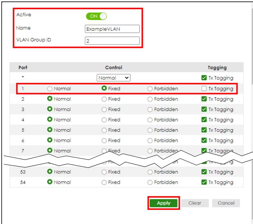
Note: The **VLAN Group ID** field in this screen and the **VID** field in the **SYSTEM > IP Setup > IP Status** screen refer to the same VLAN ID.
