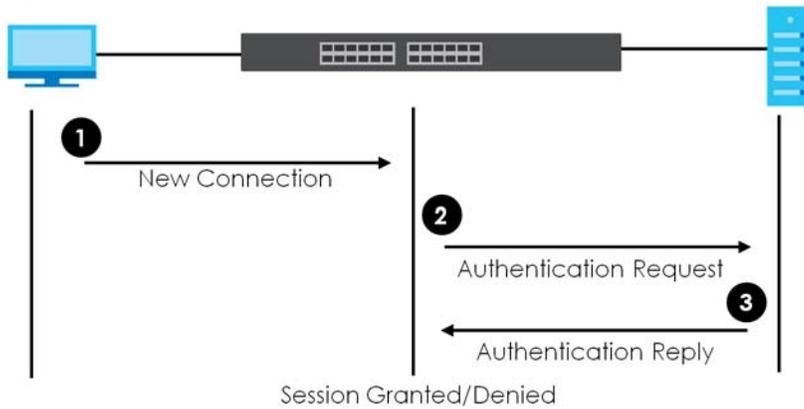
Note: To enable port authentication, first activate the port authentication methods (both on the Switch and the ports), then configure the RADIUS server settings in the **SECURITY > AAA > RADIUS Server Setup** screen.
