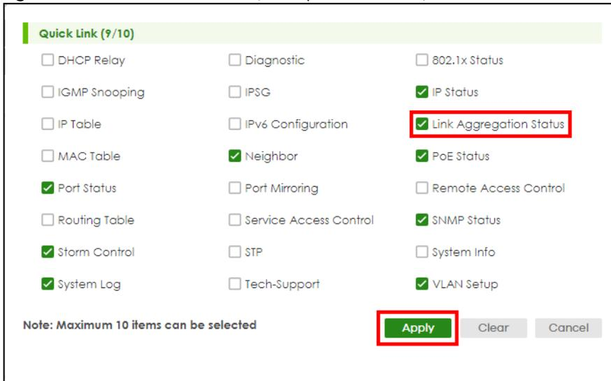
Select the quick links you want and click **Apply**. The selected quick links will be displayed in the **Quick Link** section on the **DASHBOARD** screen.
