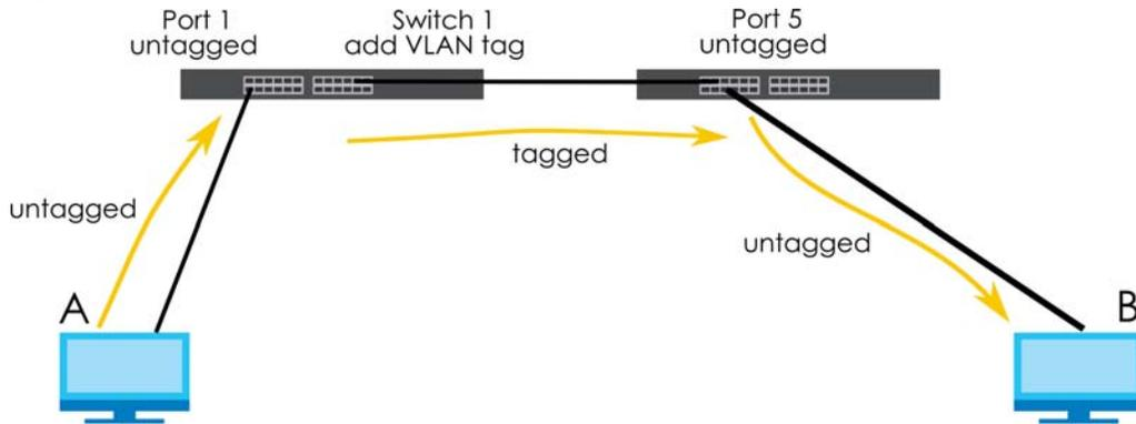
A broadcast frame (or a multicast frame for a multicast group that is known by the system) is duplicated only on ports that are members of the VID (except the ingress port itself), thus confining the broadcast to a specific domain.
