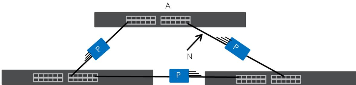
Note: After resolving the loop problem on your network you can re-activate the disabled port through the Web Configurator or through commands (See the CLI Reference Guide).
