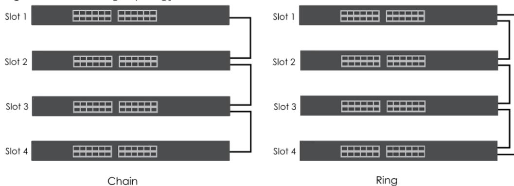
Use the master Switch to assign a 'slot ID' for each 'linecard' non-master Switch. 'Slot' refers to a Switch in the 'virtual chassis' stack.
