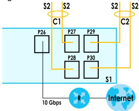
The following figure shows the connections in Switch 1 (S1) with stacking ports **P29** in Channel 1 (C1) and **P30** in Channel 2 (C2) connecting to Switch 2 (S2).
