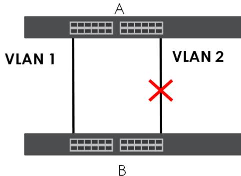
With MSTP, VLANs 1 and 2 are mapped to different spanning trees in the network. Therefore traffic from the two VLANs travel on different paths. The following figure shows the network example using MSTP.
