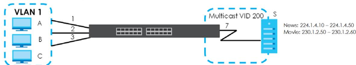
To configure the MVR settings on the Switch, click the **Add/Edit** button in the **SWITCHING > Multicast > MVR** screen. Create a multicast VLAN and set the receiver and source ports.
