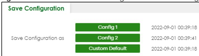
Note: If a customized default file was not saved, clicking **Custom Default** in the **MAINTENANCE > Reboot System** screen loads the factory default configuration on the Switch.
