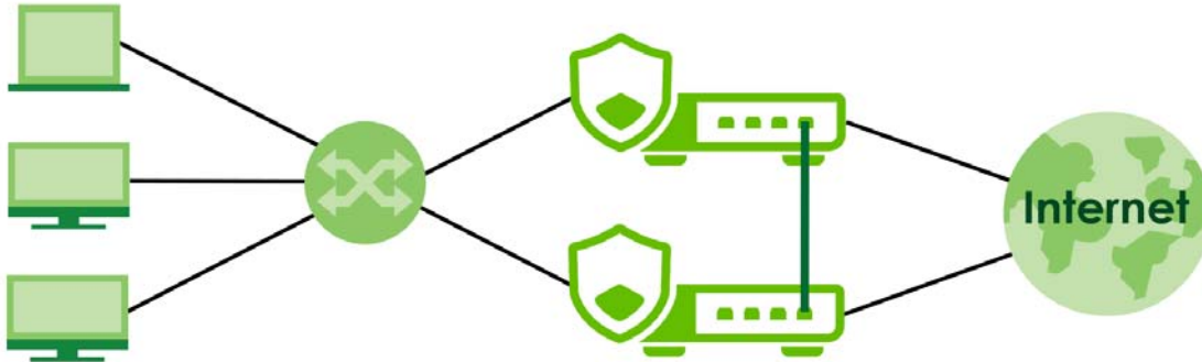
Figure 101 Device HA Backup Taking Over for the Master
